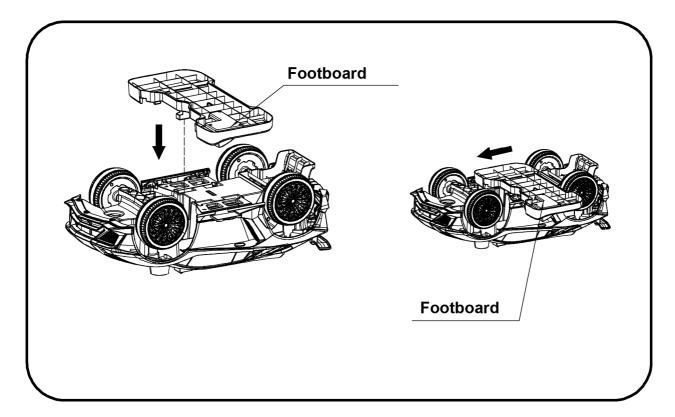
• As shown in the picture, install the footboard to the corresponding place, also push the footboard forward in the direction of the arrow and make sure to fit in position.
