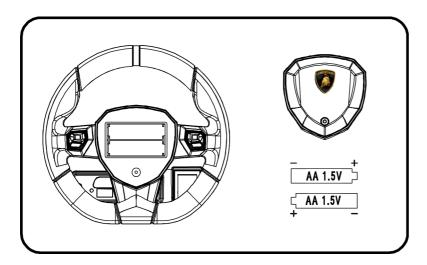
Loosen battery cover of steering wheel control and remove the cover. Insert two AA1.5V batteries(See above photo). Replace battery cover.
