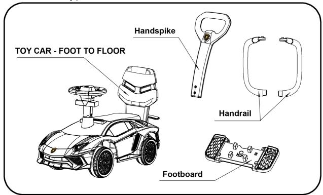
Remove the handspike, handrail and footboard from the vehicle body separately. You can turn
