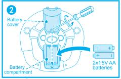
Open the steering wheel battery cover (as shown in Figure 1), find the positive pole and negative pole, and put 2AA batteries into the compartment properly, then close the battery cover and fix it with the screw (as shown in Figure 2).
